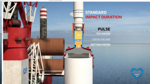
Figure 5-15. PULSE Noise Reduction System Features (Source: Included with permission from IQIP 2022b)
