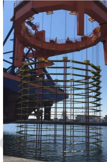
Figure 5-7. Winch Frame and AdBm System (Source: Included with permission from AdBm 2020)
