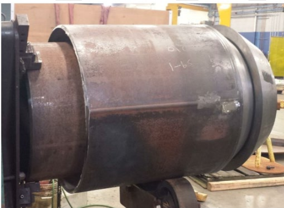
Figure 5-8. Pile Shoe Assembly for Double-wall Pile System (Source: WSDOT 2015)
