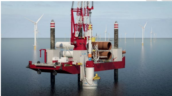
Figure 5-14. PULSE Noise Reduction System (Source: Included with permission from IQIP 2022b)
