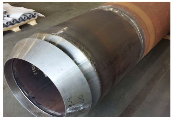
Figure 5-9. Double-wall Pile (Source: WSDOT 2015)
