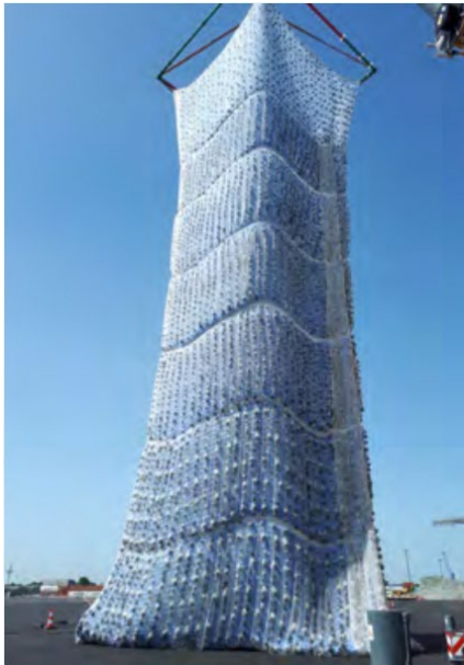
Figure 5-4. Hydro-sound Damper Net (Source: Included with permission from OffNoise 2022)
