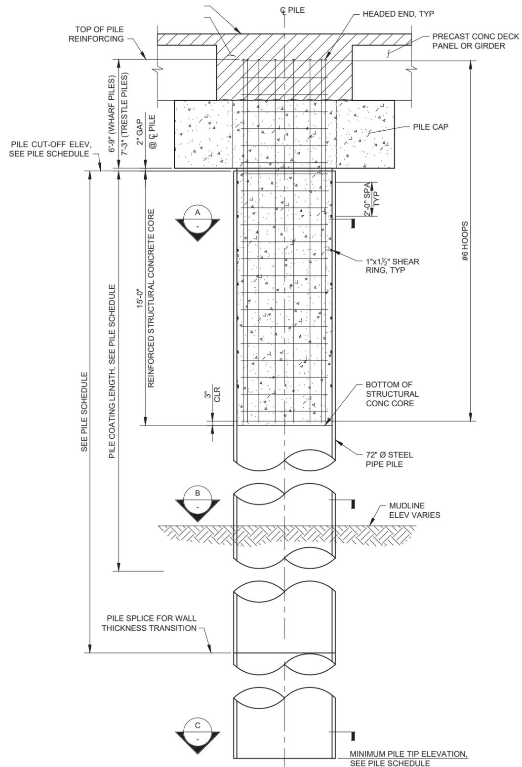
**TYPICAL PILE ELEVATION**
