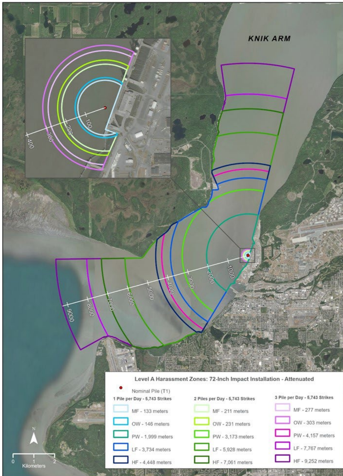
Figure 6-2. Level A Harassment Isopleths for Impact Installation of 72-Inch Piles (Attenuated) for Production Rate of One to Three Piles per Day
