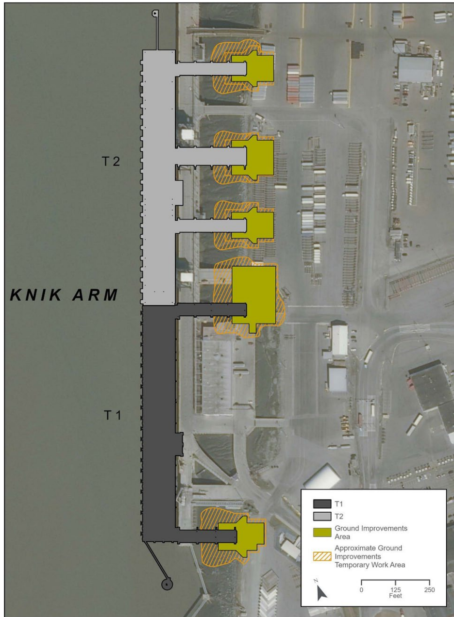
Figure 2. Component 1: Ground Improvement Locations and Approximate Areas. Image from Biological Assessment (Port of Alaska 2024).
